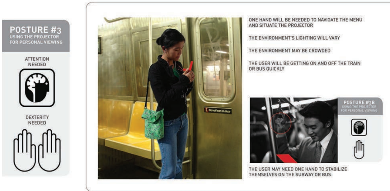
Figure 4.18 A posture study of a personal projector (from Mio, by Audrey Liu, used by kind permission of Audrey Liu).
